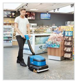
Raise the front squeegee to quickly and conveniently pick up smaller debris while scrubbing.
